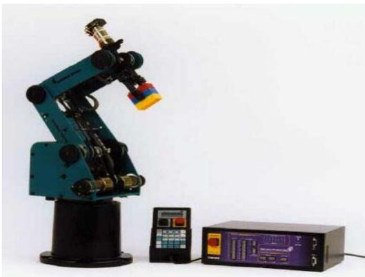
Fig 2. Robô Scorbot ER-4PC (ER4PC)
